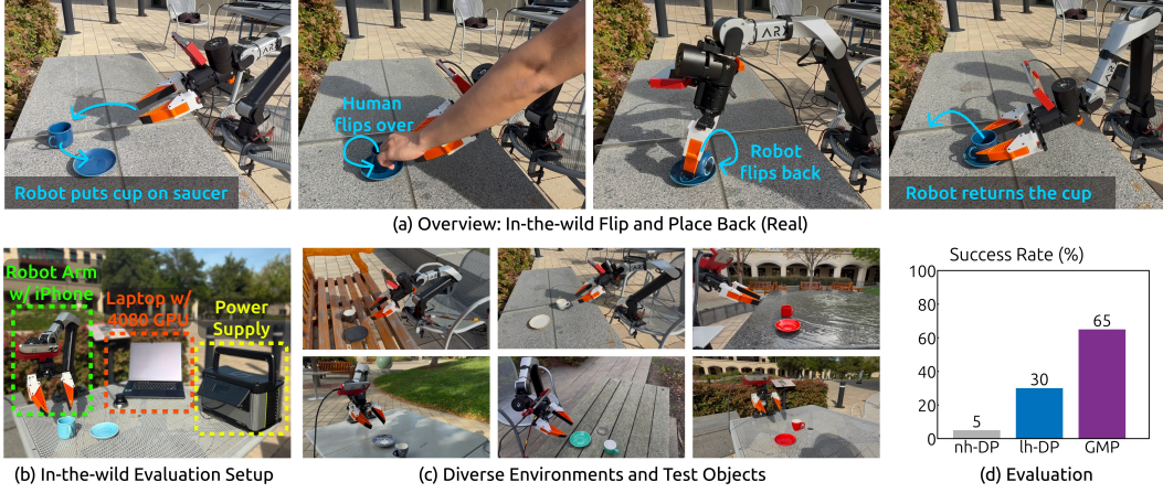
Figure 6: Task 3: Flip and Place Back (Real) . (a) After the robot picks up the cup and places it on the saucer, a human flips it over by 90 degrees. The robot must flip it back then return it to the original position. (b) We use an portable ARX X5 robot arm with an iPhone for visual observation. (c) We evaluate our policy on 6 challenging unseen environments and over 10 cups, showing robustness and generalizability across objects and scenes.
